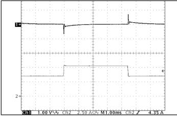
Figure 5: Output voltage response to step-change in load current (66 % -100 %-66 % of Iout(max);  $dI/dt = 0.1 A/\mu s$ ). Load cap: 15  $\mu F$  tantalum cap and 1  $\mu F$ ceramic cap. Ch 1: Vout (1 V/div), Ch 2: Iout (2.5 A/div).
