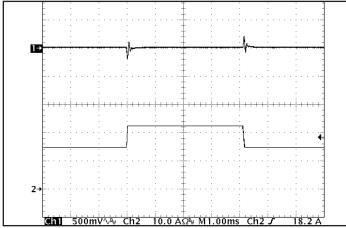
Figure 5: Output voltage response to step-change in load current (66 % -100 %-66 % of Iout(max);  $dI/dt = 0.2 A/\mu s$ ). Load cap: 15  $\mu F$  tantalum cap and 1  $\mu F$ ceramic cap. Ch 1: Vout (500 mV/div), Ch 2: Iout (10 A/div).
