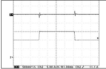
Figure 5: Output voltage response to step-change in load current (66 % -100 % -66% of lout(max);  $dI/dt = 0.1 A/\mu s$ ). Load cap: 15  $\mu F$  tantalum cap and 1  $\mu F$  ceramic cap. Ch 1: Vout (500 mV/div), Ch 2: lout (5 A/div).
