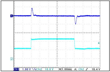
Figure 6: Output voltage response to step-change in input voltage (250 V/ms). Load cap: 100 µF electrolytic output capacitance. Ch 1: Vout (1 V/div), Ch 2: Vin (10 V/div).
