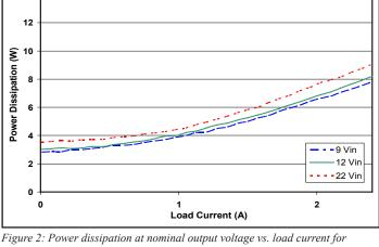
minimum, nominal, and maximum input voltage at 25 °C.
