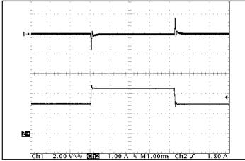
Figure 5: Output voltage response to step-change in load current (66 % -100 %-66 % of Iout(max);  $dI/dt = 0.05 A/\mu s$ ). Load cap: 1  $\mu F$  ceramic cap. Ch 1: Vout (2 V/div), Ch 2: Iout (1 A/div).
