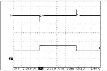
Figure 5: Output voltage response to step-change in load current (66 % -100 % -66 % of Iout(max);  $dI/dt = 0.08 A/\mu s$ ). Load cap: 1  $\mu F$  ceramic cap. Ch 1: Vout (2 V/div), Ch 2: Iout (2 A/div).
