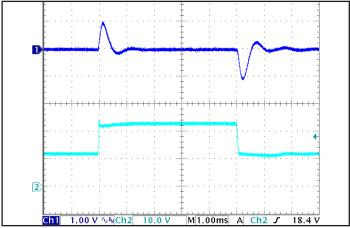
Figure 6: Output voltage response to step-change in input voltage (250 V/ms). Load cap:  $100 \mu$ F electrolytic output capacitance. Ch 1: Vout (1 V/div), Ch 2: Vin (10 V/div).
