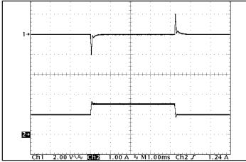
Figure 5: Output voltage response to step-change in load current (66 % -100 % -66 % of Iout(max);  $dI/dt = 0.02 A/\mu s$ ). Load cap:  $1 \mu F$  ceramic cap. Ch 1: Vout (2 V/div), Ch 2: Iout (1 Iout).
