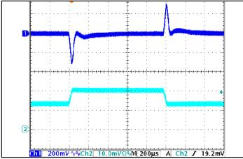
Figure 5: Output voltage response to step-change in load current (66 % -100 % -66 % of Iout(max); dI/dt = 0.1 A/ $\mu$ s). Load cap: 15  $\mu$ F tantalum cap and 1  $\mu$ F ceramic cap. Ch 1: Vout (200 mV/div), Ch 2: Iout (5 A/div).
