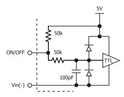
Figure B: Internal ON/OFF pin circuitry
