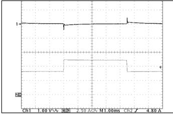
Figure 5: Output voltage response to step-change in load current (66 % -100 % -66 % of Iout(max); dI/dt = 0.1  $A/\mu s$ ). Load cap: 15  $\mu F$  tantalum cap and 1  $\mu F$  ceramic cap. Ch 1: Vout (1 V/div), Ch 2: Iout (2.5 Iout).
